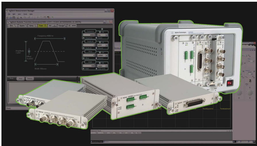
The U2700A series turns USB into a plug-in modular-instrumentation platform. The portable chassis at right, which you can also mount in an equipment rack, houses and powers the modules, which you can also connect individually to a host PC. The chassis provides facilities for synchronizing the operation of the modules it contains. Included software (background) makes short work of common functions, such as specifying waveform parameters.
