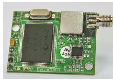
The Mini Socket iWiFi enables secure-Wi-Fi connectivity for Internet Protocol-based industrial devices over IEEE 802.11b/g networks.
